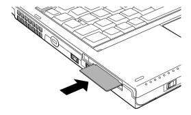
Figure 3-3 Inserting a Smart Card
